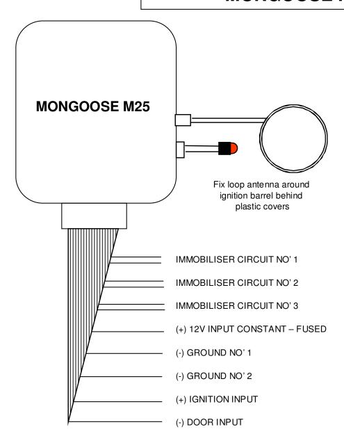
This product must be installed according to the requirements of the AS/NZS 3749.2 Installation Standard. Remove all wire identifiers during installation. Remove all wire identifier labels during installation.
